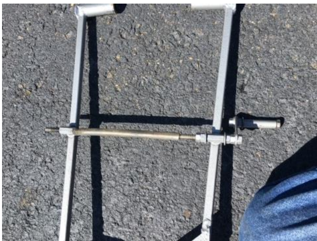
Details of the tow bar: the left leg is hinged; the threaded-rod crank allows the mechanism to be latched onto the nose gear's steering lugs.
