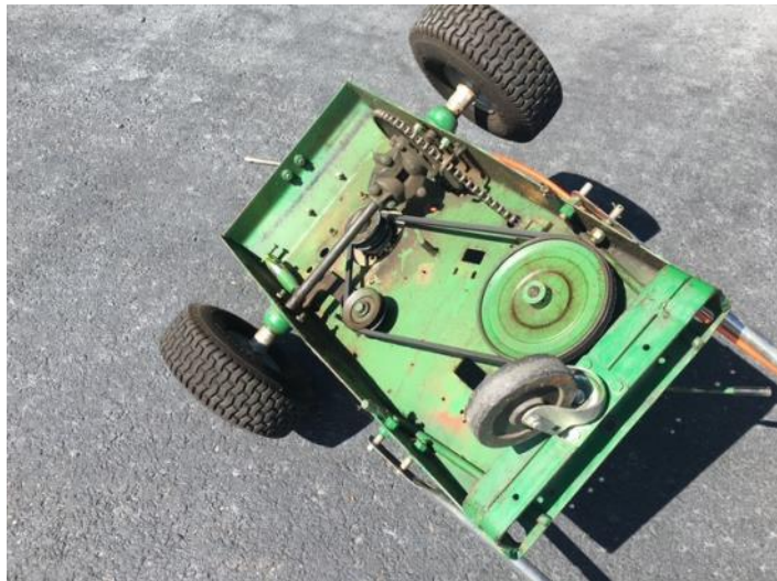
Underside of the tug, showing use of the original drive system, including a small differential on the axles. The large pulley is the input to the transmission. Also shown is the large caster wheel and its support.
